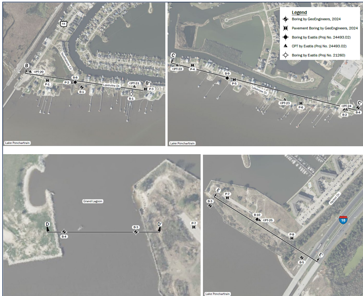
Figure 5: Borings and CPTs in Project Area
