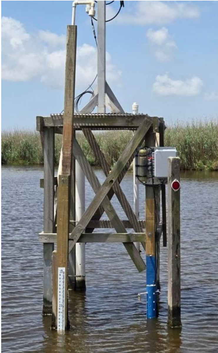
Figure F-4. Photo of CRMS2418-H02 which is mounted onto the USGS four post platform. Survey the CR and SG and be sure to indicate the station is –H02 which differentiates the site from the old USGS real-time station that was on the same platform. A new staff gauge was added when the station was set-up. Only survey the new staff gauge.
