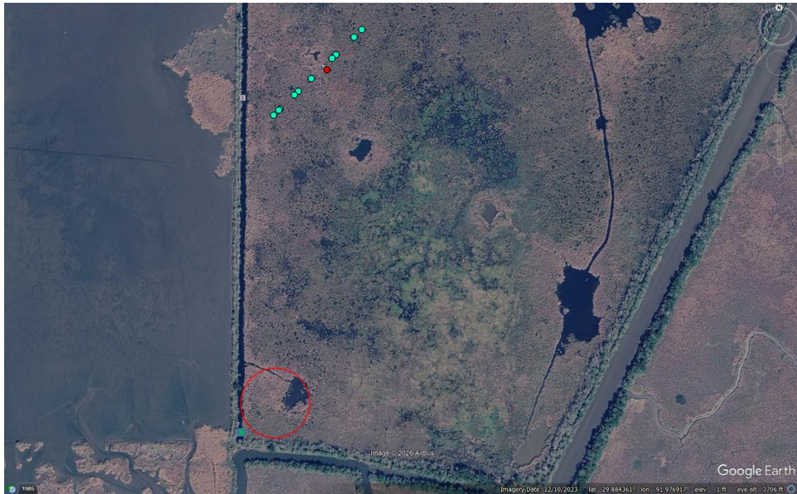
Figure B-1g. Locations where marsh elevation is to be surveyed at CRMS0511. The landowner does not allow CRMS to access the site with an airboat. The Hydro station (blue square) is accessed by walking over the levee to a small boardwalk. Vegetation elevation should be taken within reach of the boardwalk.
