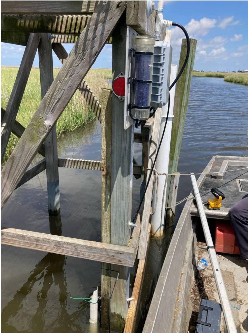
Figure F-2. Photo of CRMS0282-H02 which is mounted onto the USGS four post platform. Survey the CR and the SG and be sure to indicate the station is –H02 which differentiates the site from the old USGS real-time station that was on the same platform. Note: No new staff gauge was added when the new station was added to the platform.
