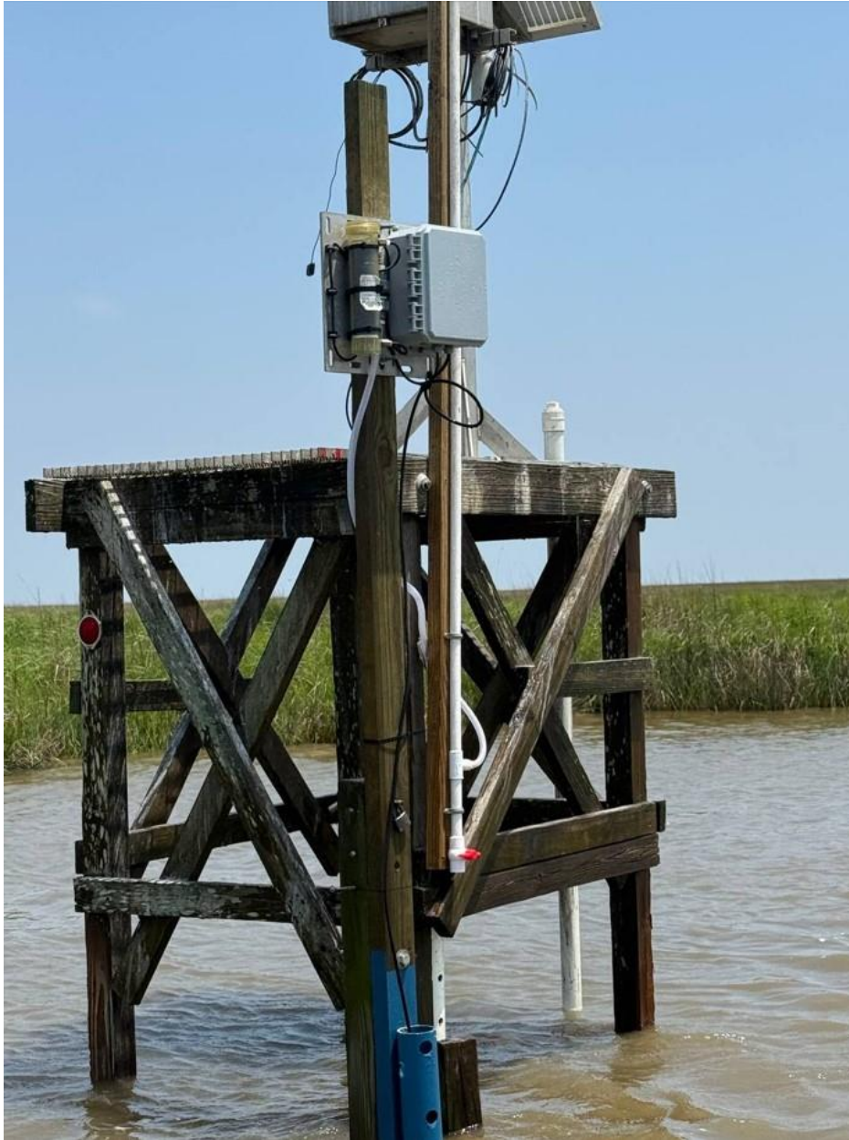
Figure F-5. Photo of CRMS0609-H02 which is mounted onto a post adjacent to the USGS four post platform. Survey the CR and SG of the active station and be sure to indicate the station is – H02 which differentiates the site from the old USGS real-time station that was on the same platform. A new staff gauge was added when the station was set-up. Only survey the new staff gauge.
