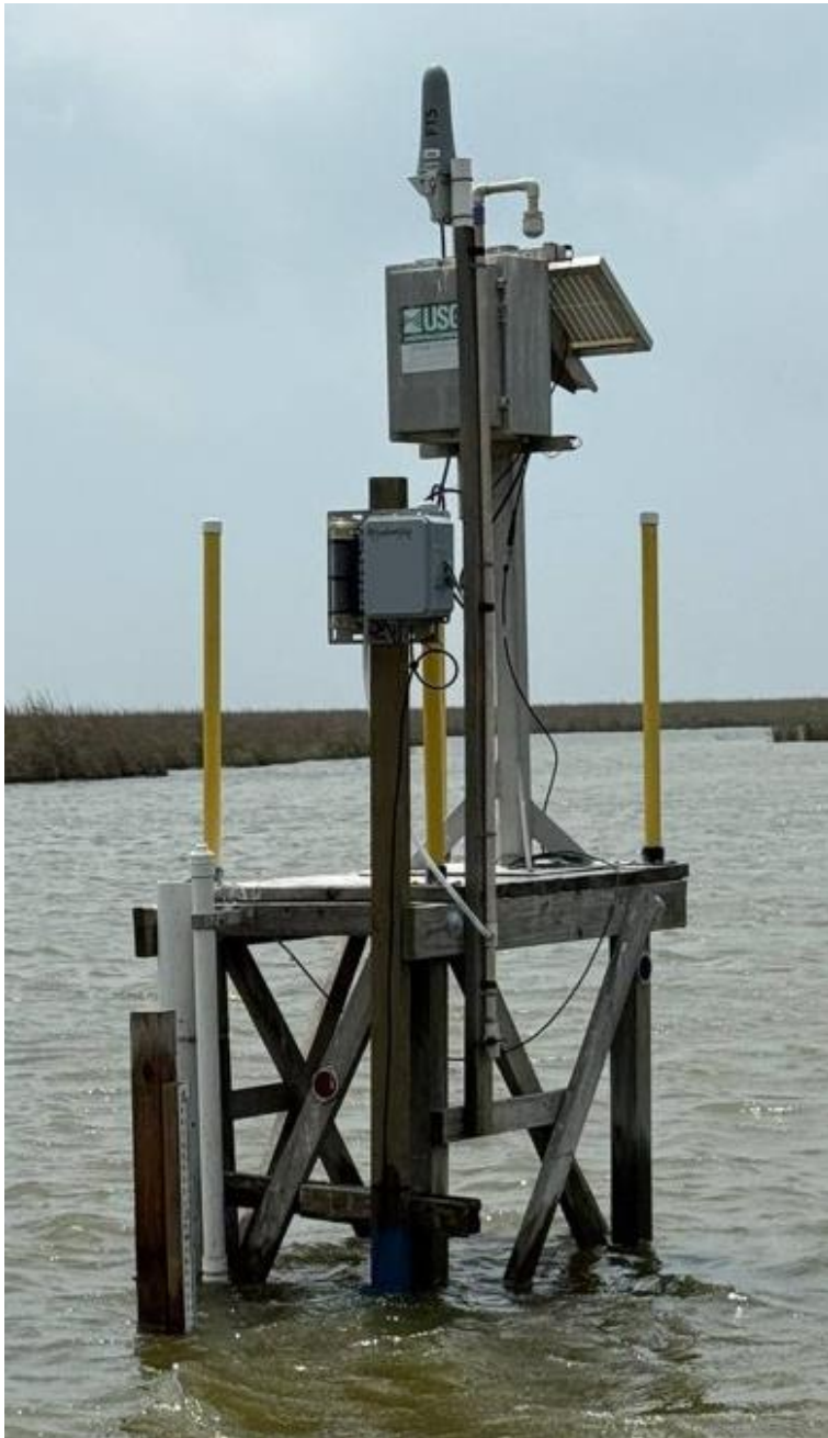
Figure F-6. Photo of CRMS0615-H02 which is mounted onto the USGS four post platform. Survey the CR and SG and be sure to indicate the station is –H02 which differentiates the site from the old USGS real-time station that was on the same platform. A new staff gauge was added when the station was set-up. Only survey the new staff gauge.
