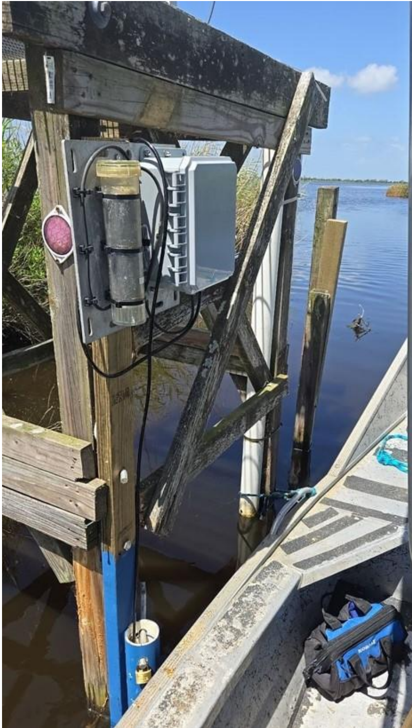
Figure F-6. Photo of CRMS0651-H02 which is mounted onto the USGS four post platform. Survey the CR and SG and be sure to indicate the station is –H02 which differentiates the site from the old USGS real-time station that was on the same platform. A new staff gauge was added when the station was set-up. Only survey the new staff gauge.
