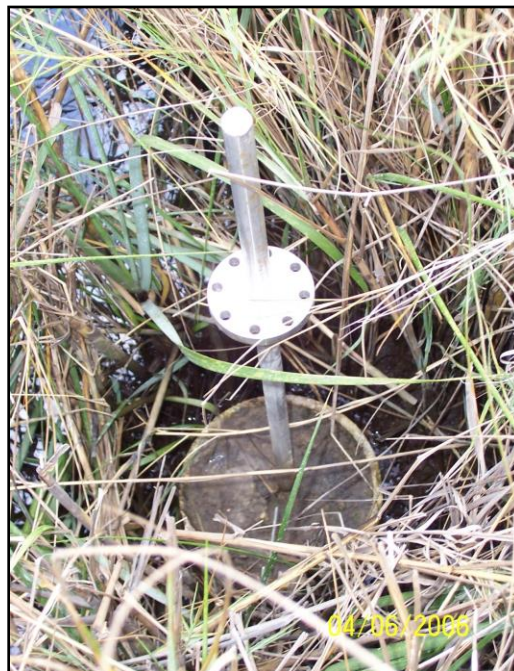
Figure A-10. Rod surface elevation table (RSET) rod and collar.
