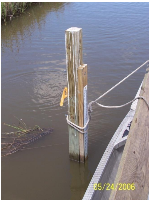
Figure A-4. Photo of a mounted staff gauge.
