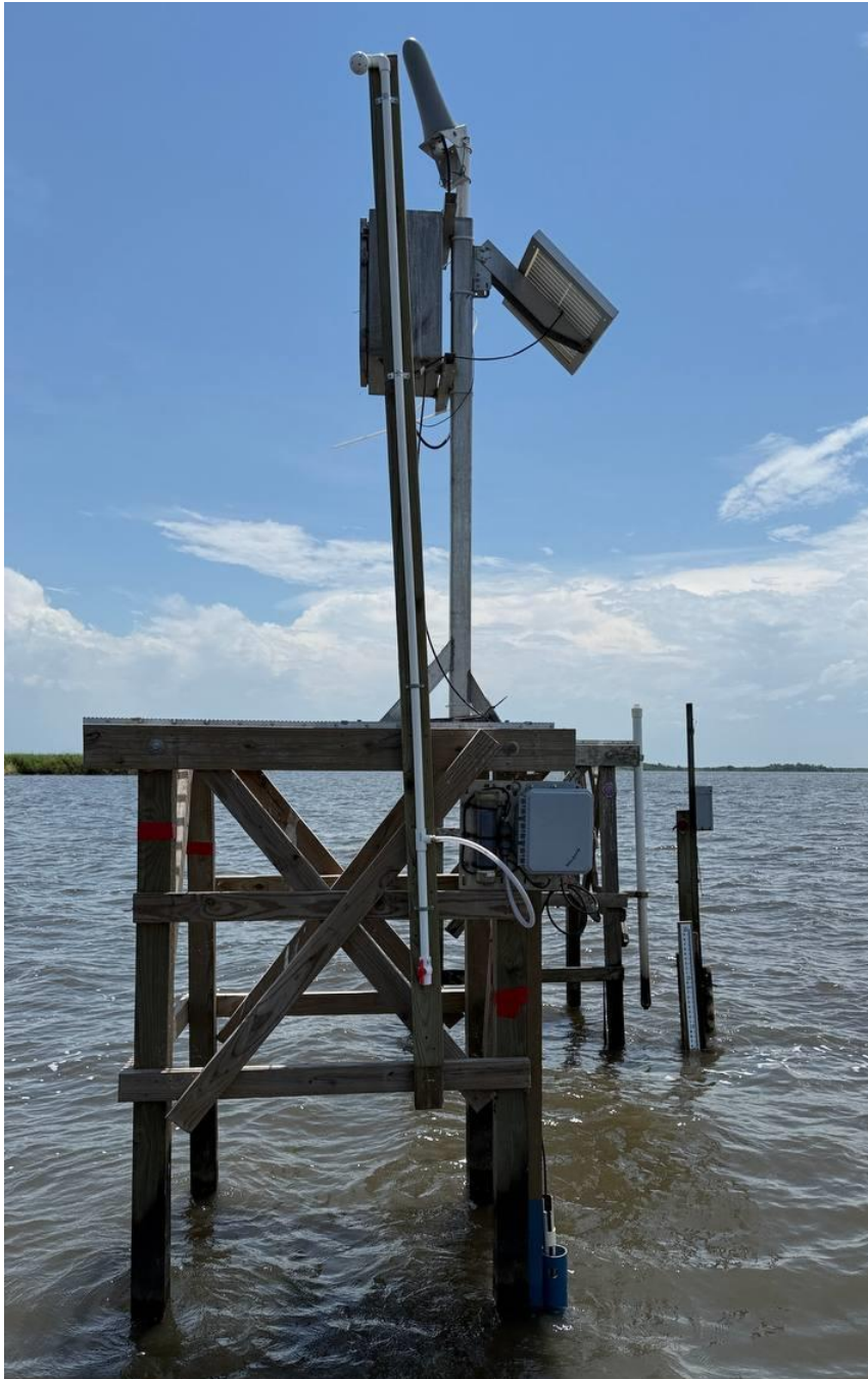
Figure F-4. Photo of CRMS0568-H02 which is mounted onto the USGS four post platform. Survey the CR and SG and be sure to indicate the station is –H02 which differentiates the site from the old USGS real-time station that was on the same platform. The current active station is the one with equipment attached to it in the foreground. A new staff gauge was added when the station was set-up. Only survey the new staff gauge.
