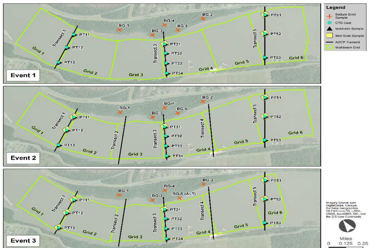
Figure 2.2. Locations of 2020 MR ADCP, bed grab and isokinetic measurement transects downstream near the Phoenix bend over the Myrtle Grove sand bar.
