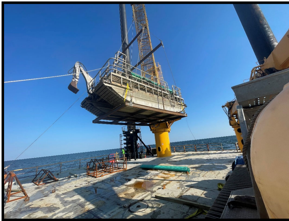
Figure 1: Marsh buggy drill being lifted into the water.
