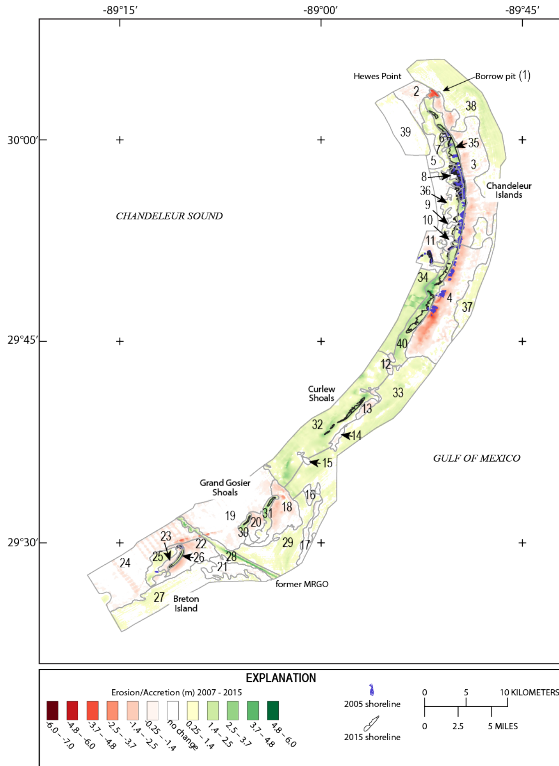
Figure 5: Chandeleur Islands 2007 to 2015 elevation change map with accretion/erosion areas identified by polygons
