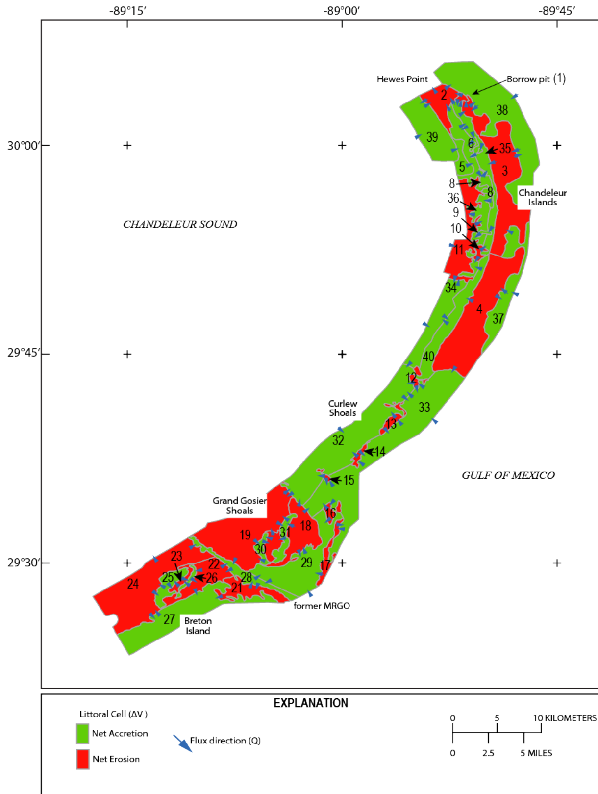
Figure 6: Littoral cells for the 2007 – 2015-time period at the Chandeleur Islands where the net volume ( \Delta V ) is positive (green) or negative (red). Blue arrows represent flux direction from (Q-source) and to (Q-sink) the cell and residual volumes are calculated to determine sediment movements and quantities.
