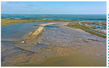
The borrow source for this project is on the east bank of the Mississippi River and subsequently across the navigation channel. To cross the navigation channel with the dredge pipe took enormous coordination with the U.S. Army Corps of Engineers, the U.S. Coast Guard, and River Pilot organizations.
