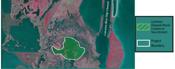
The project will also re-establish a part of the historic Long Point Bayou channel and create tidal creeks to provide tidal exchange into and out of the marsh creation area. Additionally, constructing tidal creeks will increase the marsh edge habitat, which is a highly productive transition zone between the vegetated interior of the marsh and the fluctuating intertidal zone.
