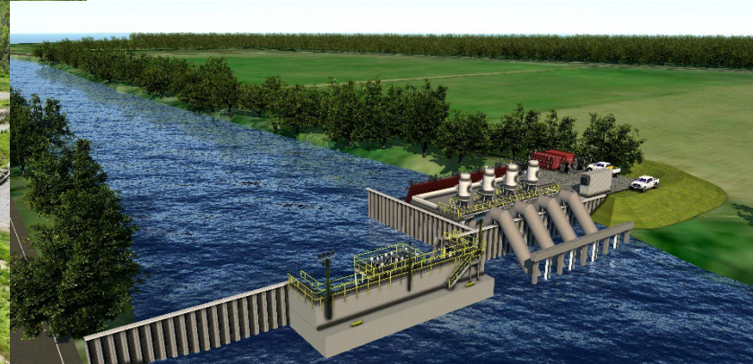
Bayou Black Pump Station 1,000 CFS Capacity In Design
