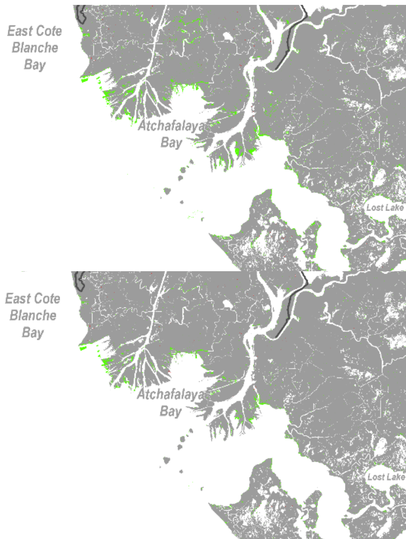
Figure D2. Zoomed in look at land area at Year 25 for test runs G021 (top) and G022 (bottom) vs. the base run, G400, for the Wax Lake area. Green indicates more land with the G021 than the G400. Red indicates the G400 model test run had land in an area which is not land in the test run. Refer to Figure D1 for scale.
