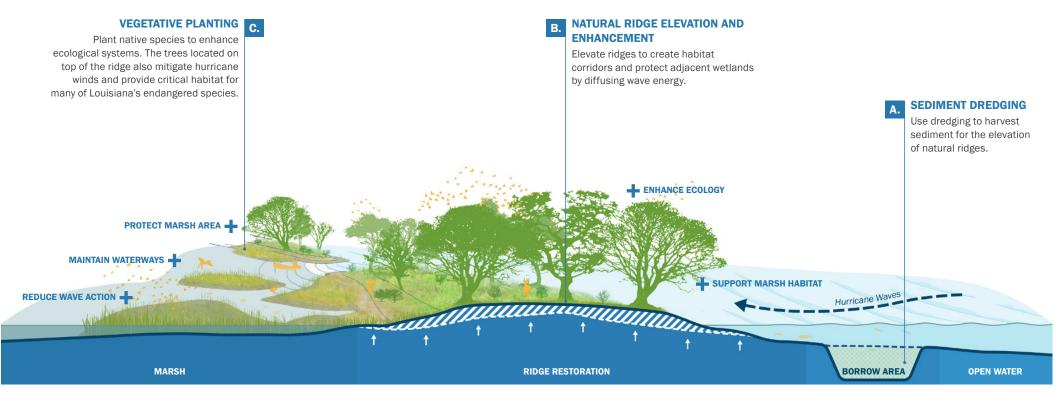
Figure 4.3: Ridge Restoration Project Type Visualization.
