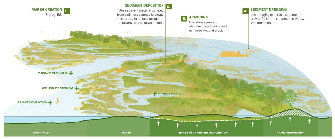
Figure 4.5: Landbridge Project Type Visualization.
