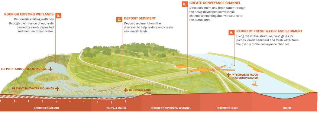
Figure 4.6: Diversion Project Type Visualization.
