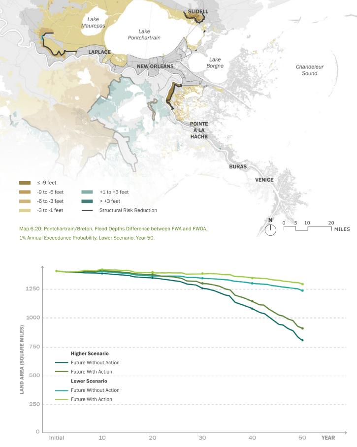
Figure 6.23: Pontchartrain/Breton Land Area Over 50 years, Future With and Without Action, Higher and Lower Scenario.
