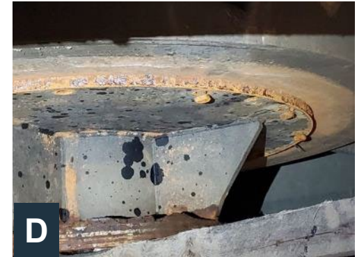
A. 1,800 pump cross section B. Diffuser section removal C. Lower diffuser bearing housing with missing bolts D. Lower diffuser bearing housing with loose bolts E. Lower bearing housing with corrosion and edge loss
