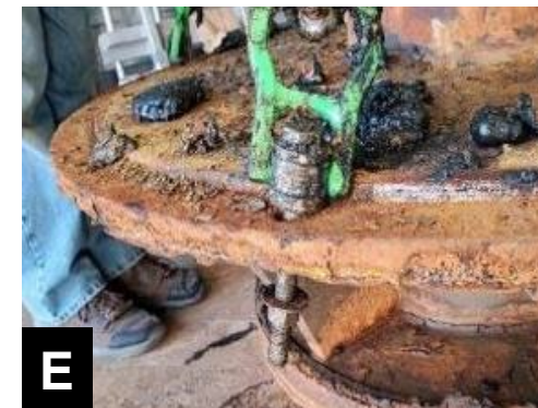
A. 1,800 pump cross section B. Diffuser section removal C. Lower diffuser bearing housing with missing bolts D. Lower diffuser bearing housing with loose bolts E. Lower bearing housing with corrosion and edge loss
