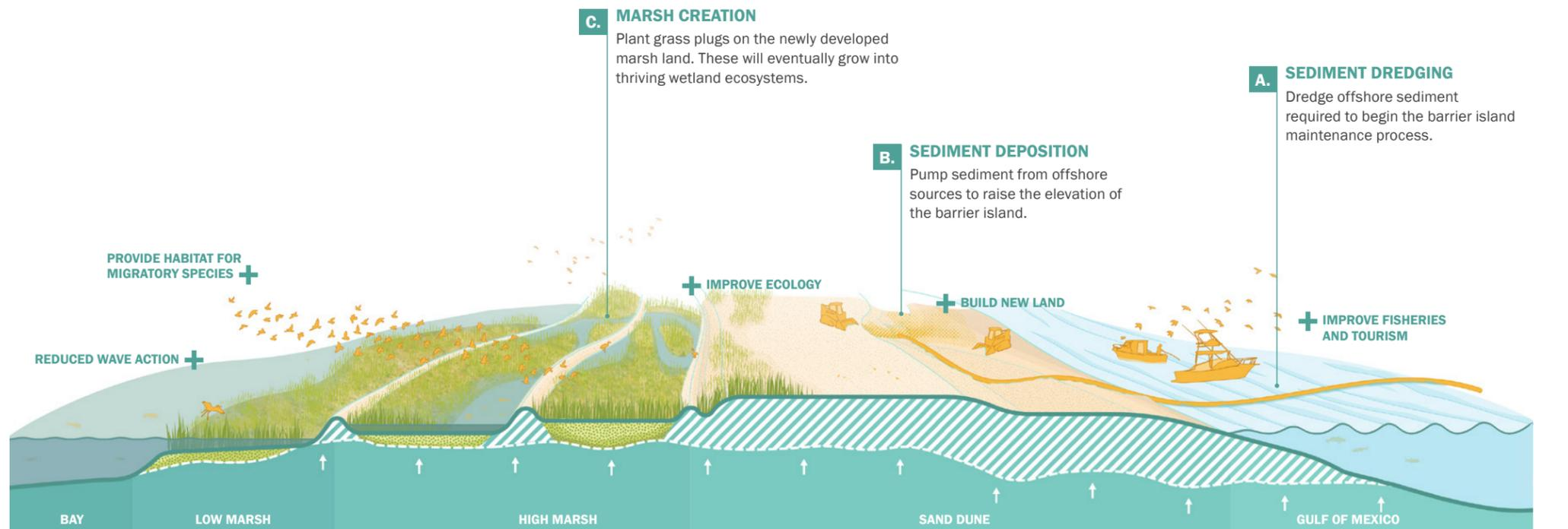
Figure 4.8: Barrier Island Maintenance Project Type Visualization.
