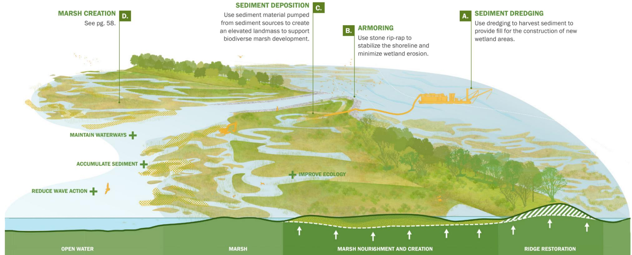
Figure 4.5: Landbridge Project Type Visualization.
