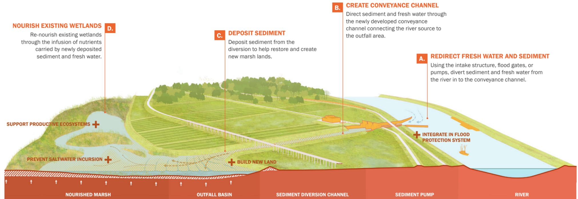
Figure 4.6: Diversion Project Type Visualization.
