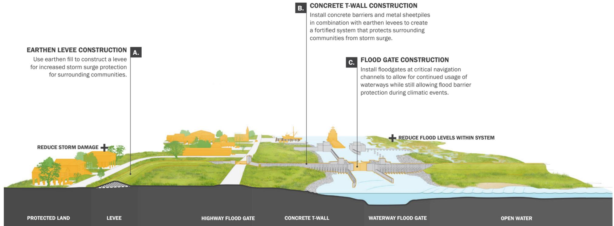
Figure 4.1: Structural Risk Reduction Project Type Visualization.
