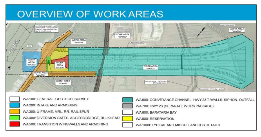
The Project's sediment delivery system is a three-component system which includes sediment intake, conveyance, and discharge.
