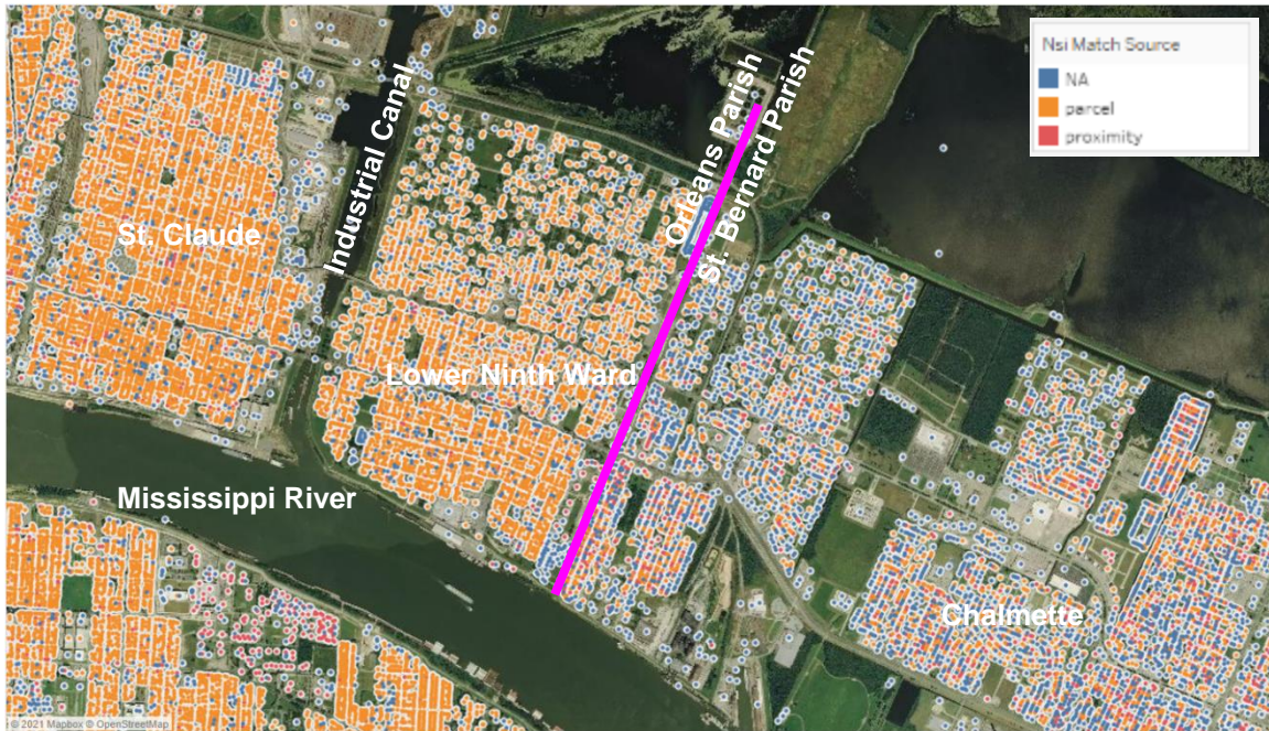
Figure 12. USACE National Structure Inventory matching methodologies near the confluence of Mississippi River and Industrial Canal. St. Claude and Lower Ninth Ward are in Orleans Parish at left, whereas Chalmette at right is in St. Bernard Parish. Orange represents where GSV and NSI structures are located within the same parcel, red where GSV and NSI structures are within 15m of each other. Because NSI structures are located along the street edge in St. Bernard Parish, the polygonal and proximity matching were unable to produce a match (in blue).
