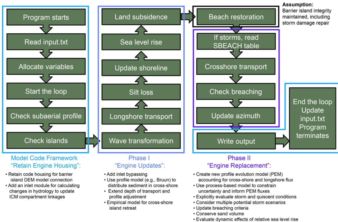
Figure 2. Suggested modifications to the BIMODE flow diagram.
