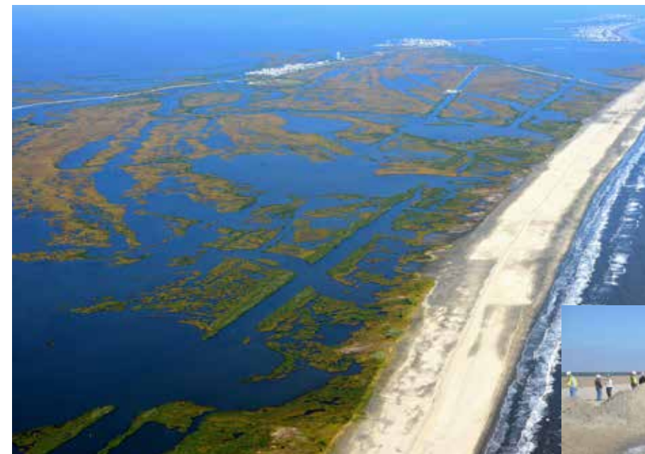
To restore the 13 miles of headland, CPRA used more than 8.4 million cubic yards of sand to create 1059 acres of beach and dune, roughly an area equivalent of almost 1047 football fields.
