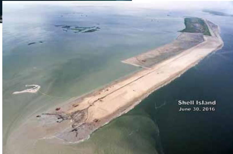
*The extension of Shell Island is seen here as the beach and dune are extended to the west using sand dredged from the Mississippi River and pipelined more than 20 miles to the site. The back marsh is also being extended to the west.*
