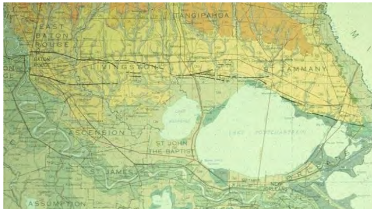
Figure 8: Official state geologic map with active Baton Rouge–Denham Springs Fault system in black.
