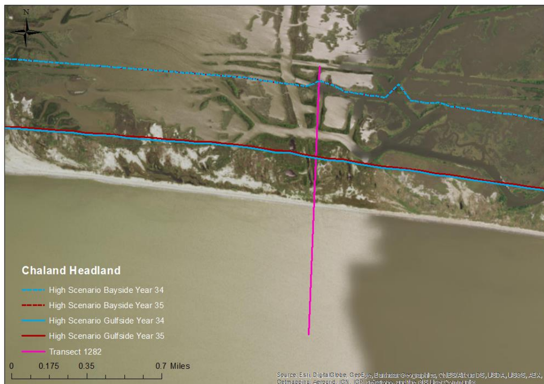
Figure 225: Plan View of Pre- and Post-Storm Shorelines for Chaland Headland at Years 34-35 with Project Implementation.
