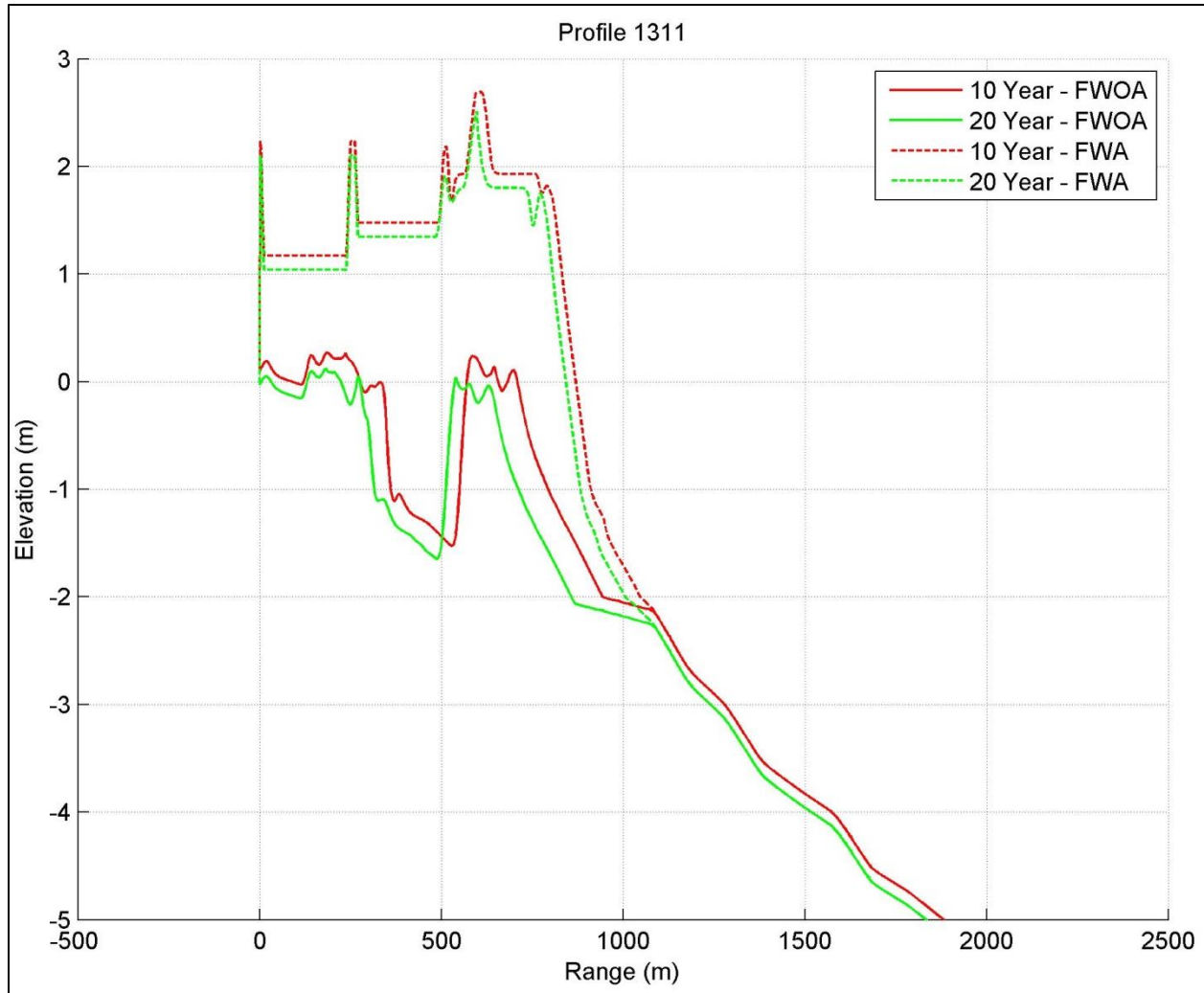
Figure 228: Representative Cross Sectional Comparison of Central Chaland Headland through Year 20 for FWOA and with the Project (FWA).
