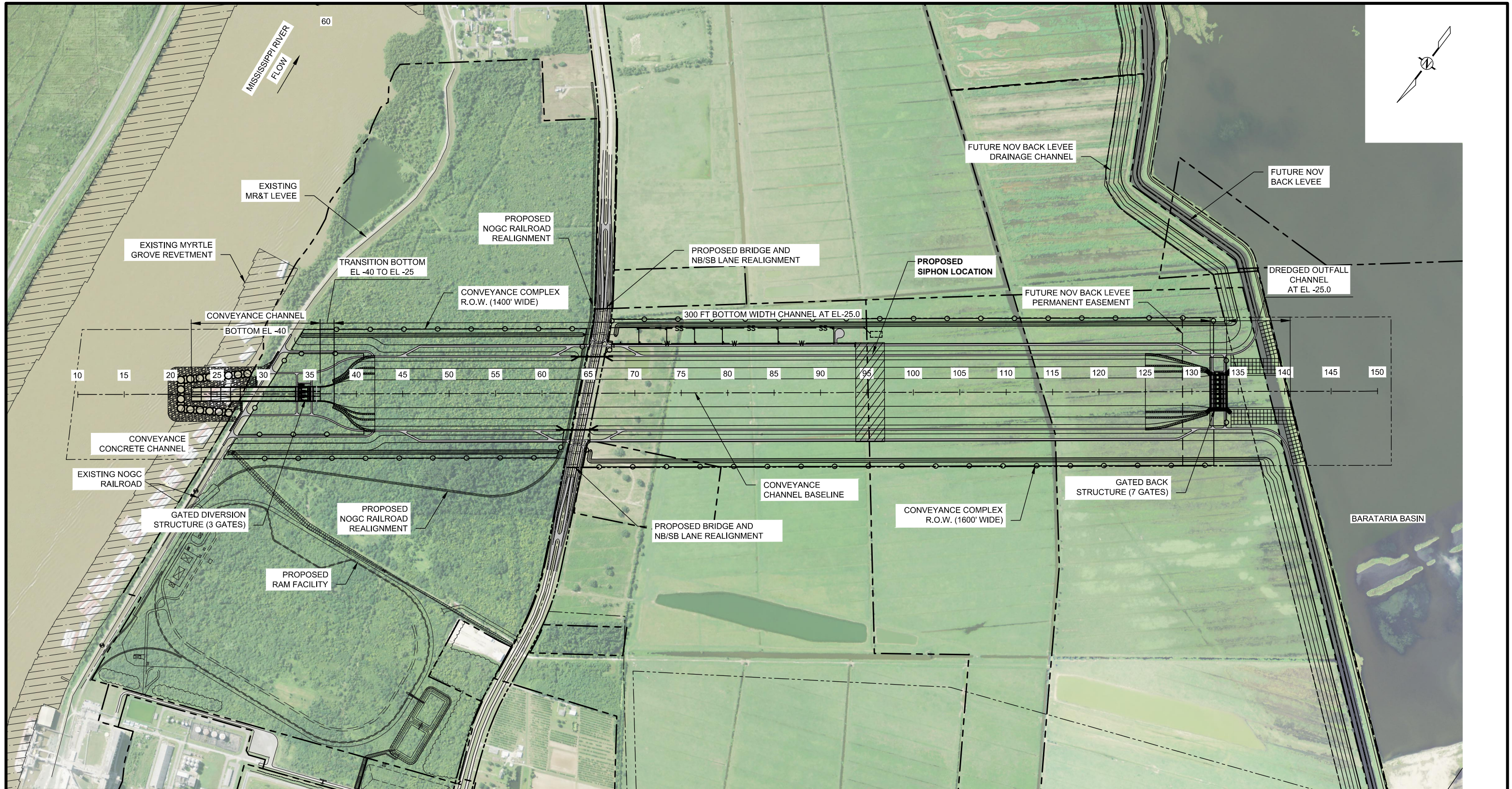
CONVEYANCE CHANNEL SITE PLAN SCALE: 1" = 1000'
