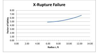
For soil below elev. -65 ft., use  $\phi = 39^{\circ}$  and  $\Upsilon = 128$  pcf. G = A $\gamma$  A = [(R<sup>2</sup> - r<sup>2</sup>)/4\*tan  $\phi$ ] - B\*y/2
