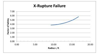
Factor of Safety for failure below cell fill:
