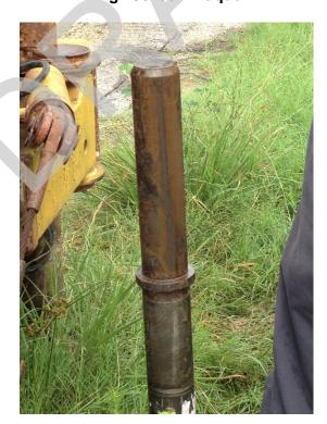
**Striking Surface Attachment to Instrumented Rod**
