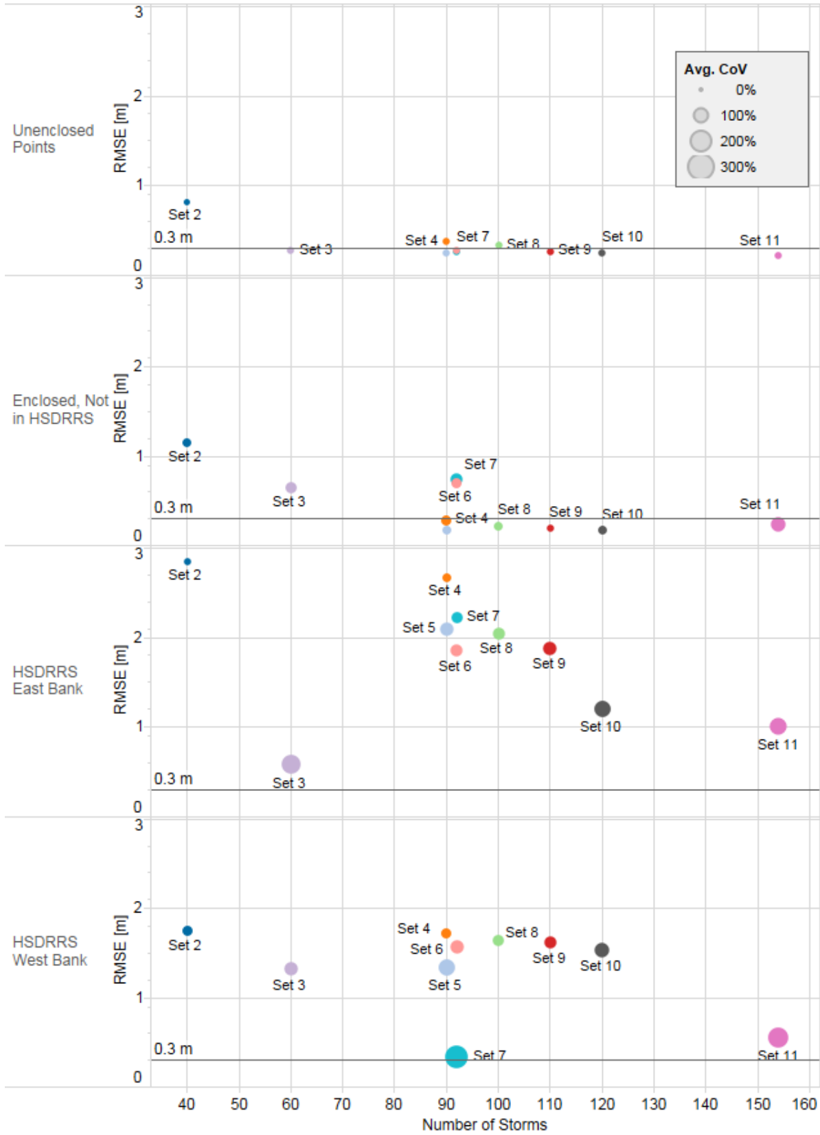
Figure 6-11: Average Bias and Variation, 500-Year Flood Depths (All Points, Split by Location).
