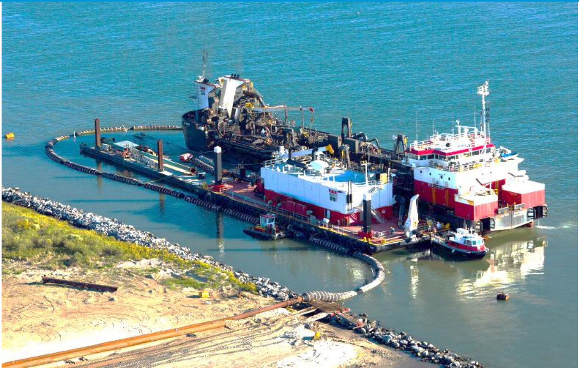
R.N. Weeks moored alongside booster pump at pump-out site on Calcasieu Channel
