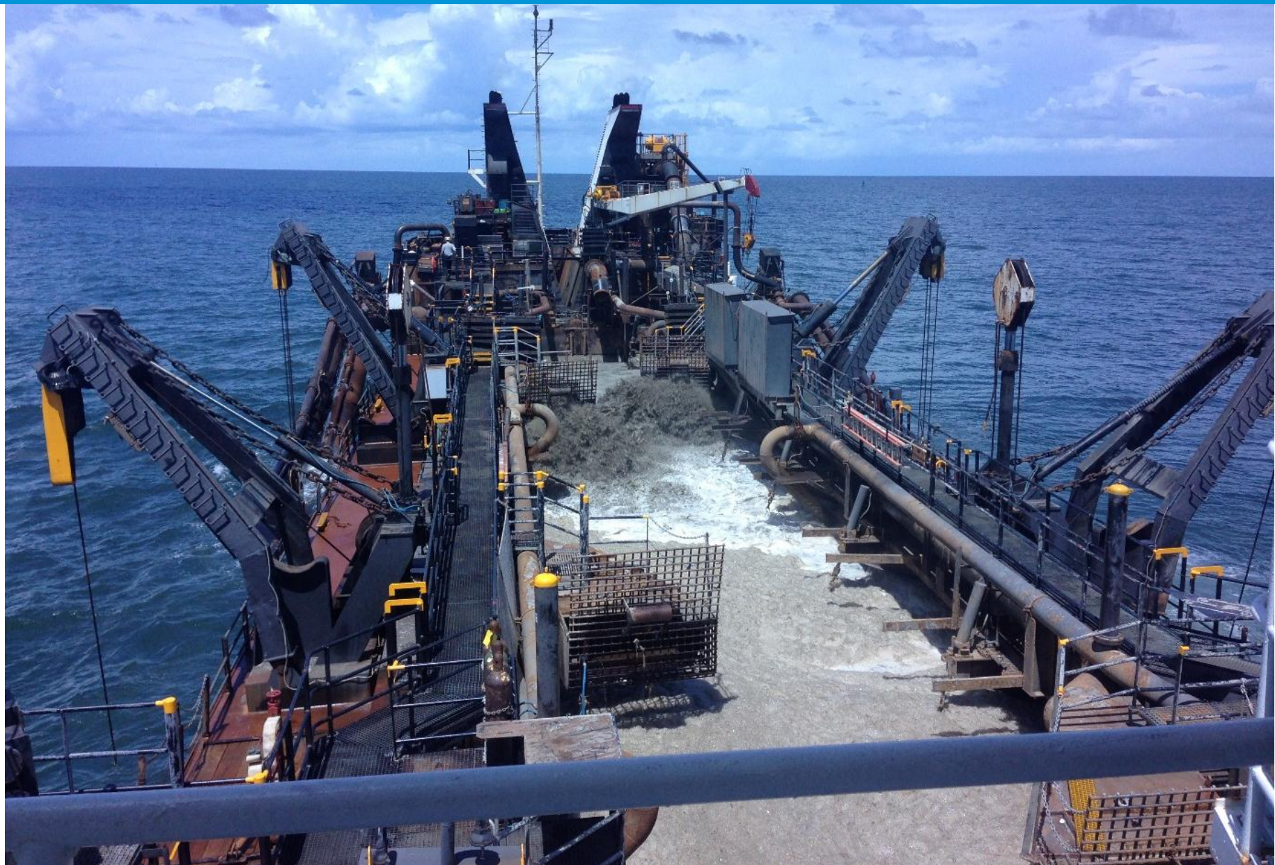
R.N. Weeks being loaded with dredged sand while at sea over borrow site.
